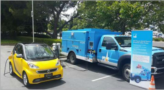
**The exportable power module on PG&E's Class 5 PHEV utility work truck is capable of providing up to 120 kW of exportable power, enough to power 80 percent of the transformers in PG&E's service area.**
